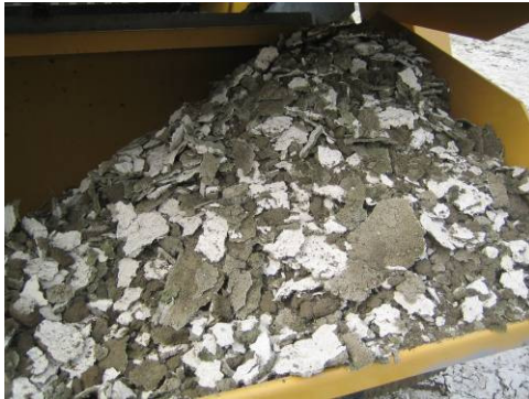
Using a small hole sized screen, the crust of the sediment can be loaded while the fines are returned to the bed.
