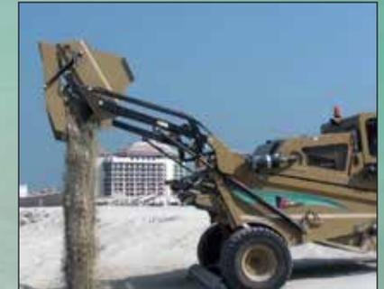
The Model 5500's clam-style hopper can be dumped to the ground or lifted to 102" (2600mm) for unloading into trucks.
