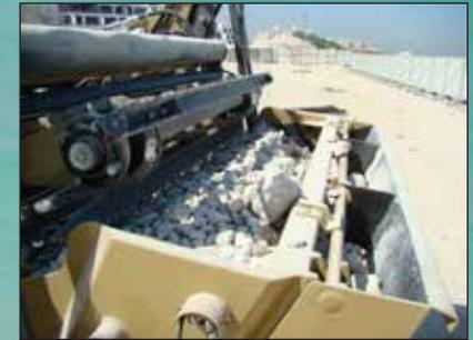
The standard hopper size is 1.5 yd<sup>3</sup> (1.2 m<sup>3</sup>) hopper. A larger, 1.8 yd<sup>3</sup> (1.4 m<sup>3</sup>) hopper, is available as an option.
