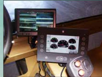
Model 5500 is equipped with screen bed/conveyor system view and backup view cameras to give the operator optimum visibility during operation.
